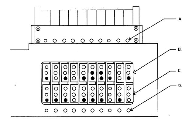
A. Splitter Screws B. Raising Changer Arm C. Lowering Changer Arm
